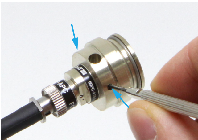
Figure 2 left: Fasten/unfasten the pin screws
