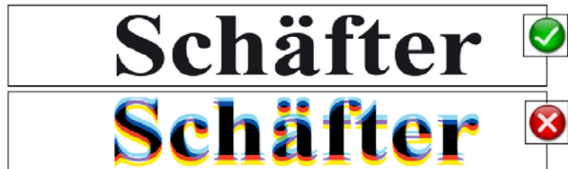
Fig. 36: Monochrome font pattern with line synchronous object pattern (good) and asynchronous transport of the object (bad - causes color convergence aberration)
